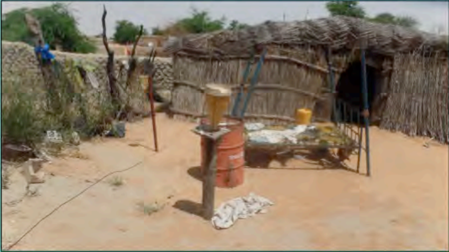
Example of a rain-gauge in northern Niger, with readings done by herders (unpaid, on a voluntary basis). In bad shape, the rain gauge is situated within the bounds of a concession, which can contribute to skewed readings, as the gauge should rather be sited in an open space, away from buildings.
